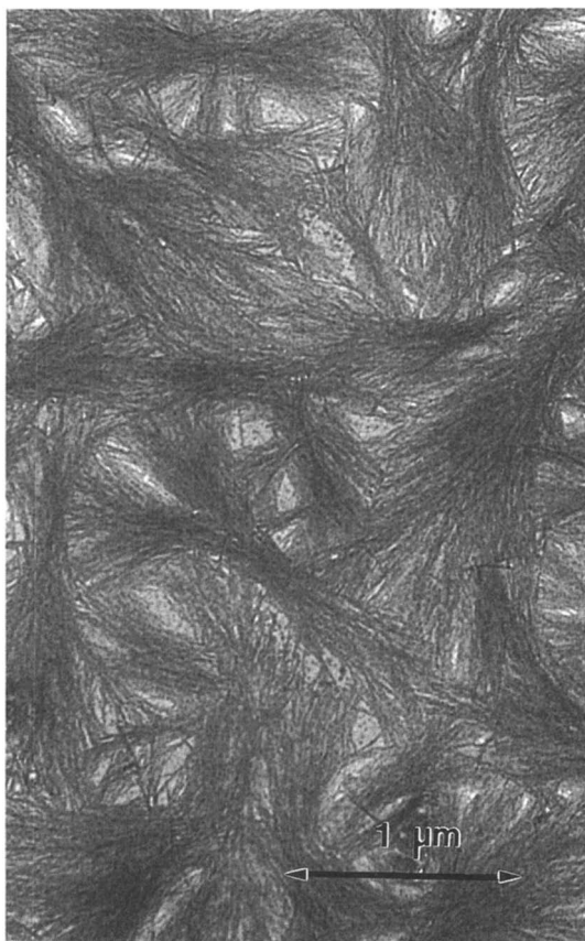
Figure 5. TEM micrograph showing spherulitic structure of SLPF similar to that commonly seen in thin films of semi-crystalline synthetic polymers.
