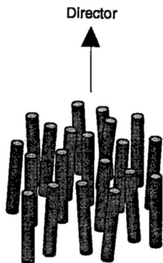
Figure 1. Illustrating local order of rod-like structures in a nematic liquid crystal, and defining the nematic director.
